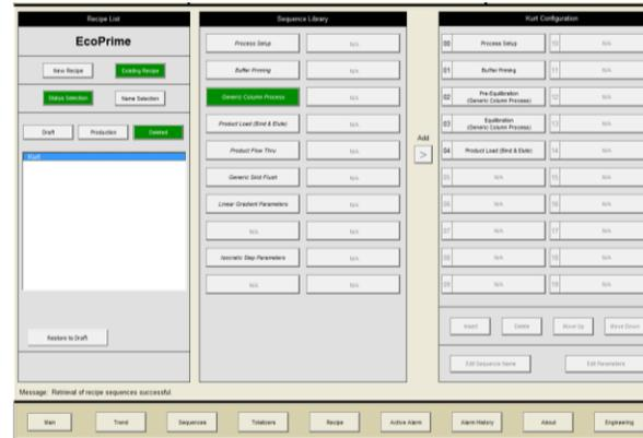
Fig 6. EcoPrime Twin LPLC Recipe configuration screen
